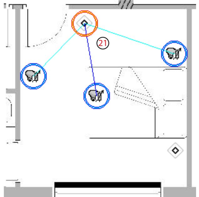
And one can go on for the other push buttons. With the push button right below, one can simply turn off all the lights by granting, one by one, the action „Off” to the three circles of light. Hereafter follows how various scenes are set.
