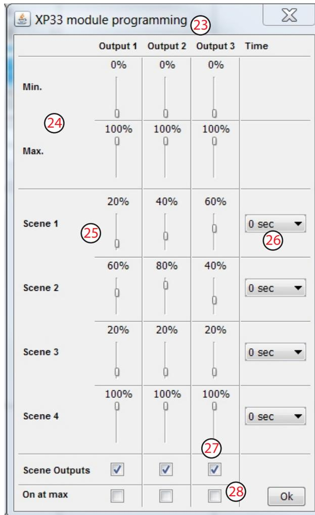
The different scenes (25) from 1 to 4 can be set with the sliders of the 3 outputs. In our example of the bedroom, scene 1 was assigned to the middle button. Adjust the sliders so in accordance with the result that gives the best impression when entering the bedroom.
