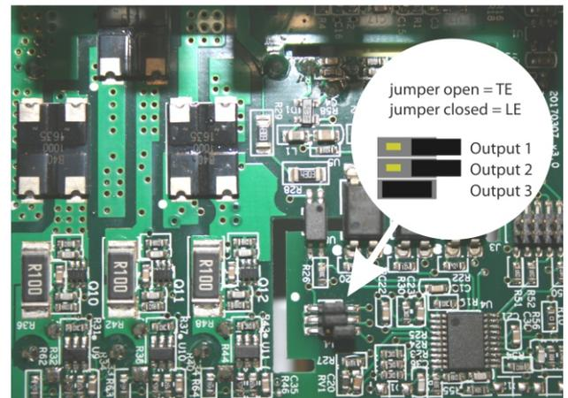
The dimmers XP33LED have the following factory setting: All 3 outputs are set for loads that require phase cut-off (TE-trailing edge). In this mode, 95% of the available LED lamps can be dimmed, notwithstanding that the load would be of a different type. If it appears that the lowest level is unstable when dimming, switch the relevant output to LE (leading edge). For inductive loads, it is recommended to use the XP33LR dimmer.
