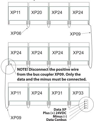
**Note:** The number of power supplies in a system is dependent on the number and the type of modules. Rule of thumb is 10 relay modules for one XP11. The software Contool determines automatically the number of power supplies.
