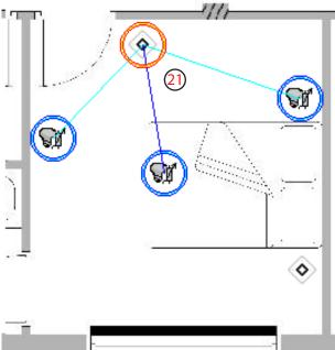
And one can go on for the other push buttons. With the push button right below, one can simply turn off all the lights by granting, one by one, the action "Off" to the three circles of light. Hereafter follows how various scenes are set.
