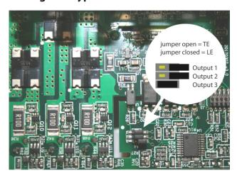
The dimmers XP33LED have the following factory setting: All 3 outputs are set for loads that require phase cut-off (TE-trailing edge). In this mode, 95% of the available LED lamps can be dimmed, notwithstanding that the load would be of a different type. If it appears that the lowest level is unstable when dimming, switch the relevant output to LE (leading edge). For inductive loads, it is recommended to use the XP33LR dimmer.
