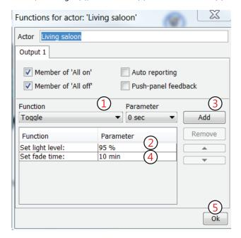
To fade downwards, take another push-button, and perform the same routine, but then to a level of light that is smaller, for example, 20% (6). To fade downwards and then completely off, add an action line Off (time): 10 min (7). Remark: The fade-time is the time to go from 0% to 100%. When the dimmer is set at 50% and one ask to go up to 100%, dimmer at 50% to 100% and asks to go, then the duration of the fade-time only is one half.
